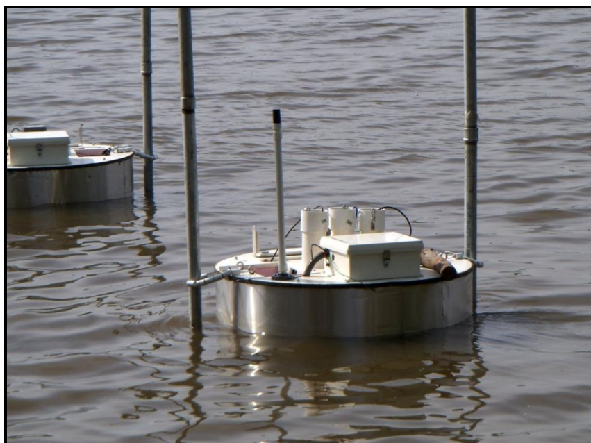
Figure 4.20: Example of sensor cluster buoy used to measure nitrate concentration located in mussel bed.
